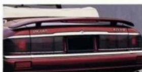
The high mount stop lamp is incorporated into the rear spoiler of 6.0L models.
