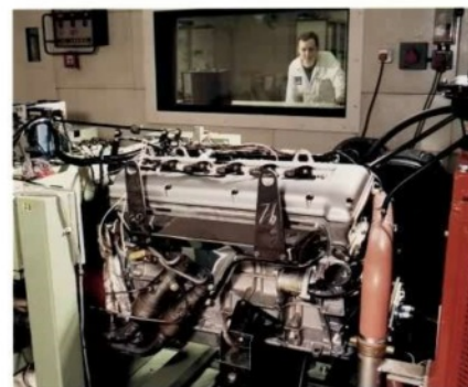
Testing on the engine dynamometer verified the durability of the new 237hp AJ16 engine.
