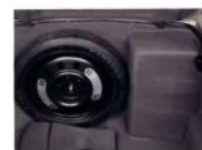
The space saver tire is now mounted on a steel wheel. (Shown with cover removed.)
