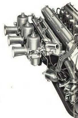
The engine fitted to the “S” type “straight port” cylinder head with three HD8 SU carburetors, a ratio, gives a power output of 250
